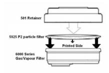
NOTE: The 5925 filter should be installed with the printed side down i.e. facing the gas filter and the clear side facing out. This allows details to be read even after use. It also provides improved service life as the non printed side has a top layer designed to reduce clogging.
